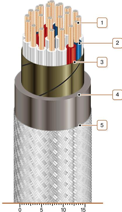
1. Copper multiwire conductor
