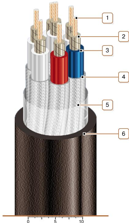
1. Copper multiwire conductor
