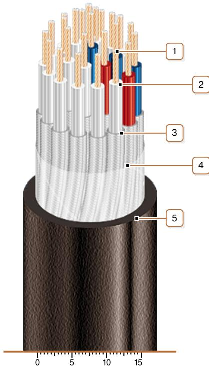
1. Copper multiwire conductor
