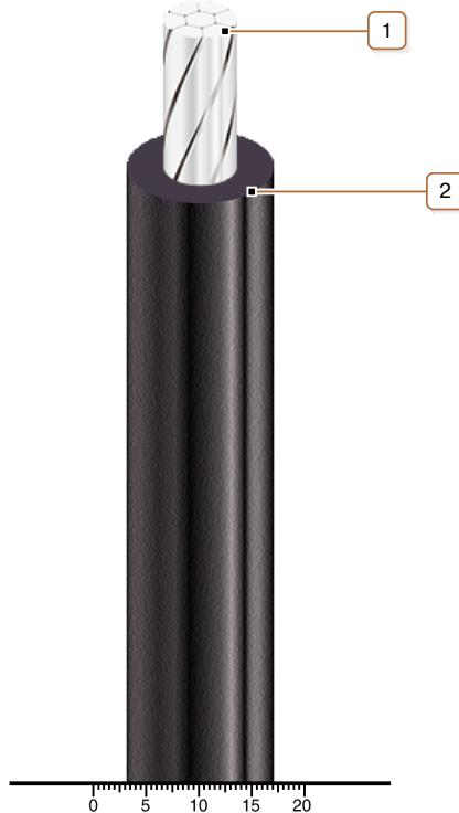
**1. Multiwire aluminium-alloy compacted conductor***Note: It is possible to manufacture the wire with longitudinal core sealing by water-blocking materials***2. Flame-retardant polymer compound insulation**
