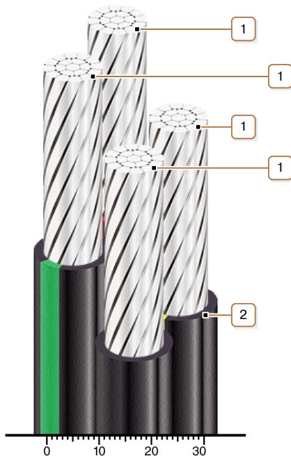
**1. Aluminium multiwire compacted conductor***Note: It is possible to manufacture the wire with longitudinal core sealing by water-blocking materials***2. Light-stabilized cross-linked polyethylene insulation***Note: Wire lay-up is not illustrated.*
