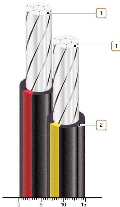
**1. Aluminium multiwire compacted conductor**
