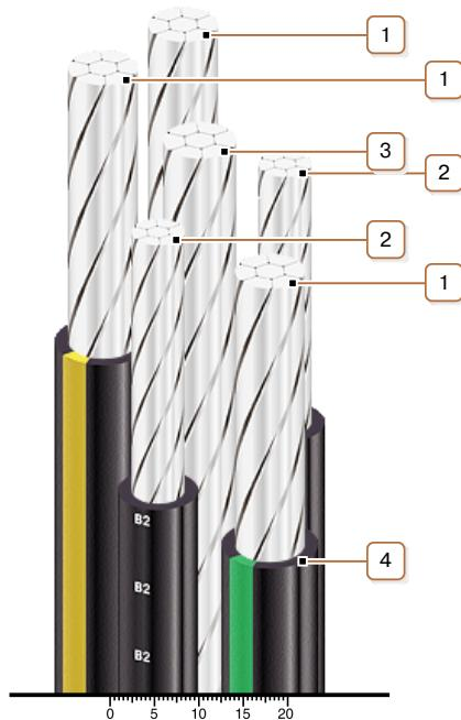
**1. Aluminium multiwire compacted conductor**
