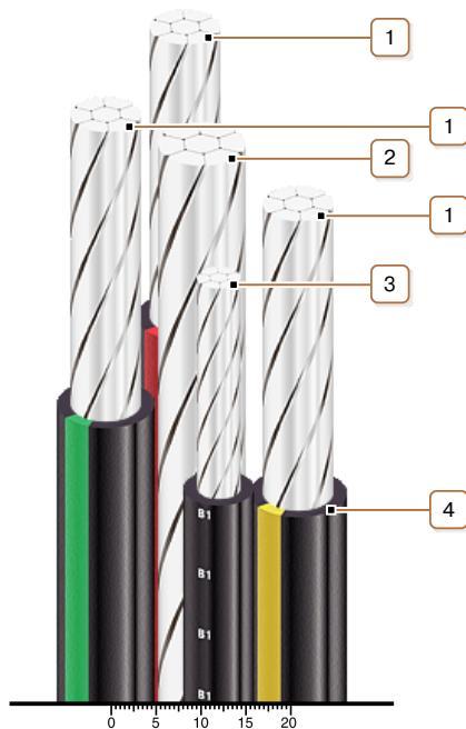
**1. Aluminium multiwire compacted conductor**
