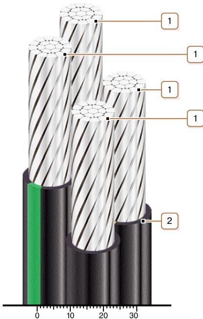
**1. Aluminium multiwire compacted conductor***Note: It is possible to manufacture the wire with longitudinal core sealing by water-blocking materials***2. Flame-retardant polymer compound insulation***Note: Wire lay-up is not illustrated.*
