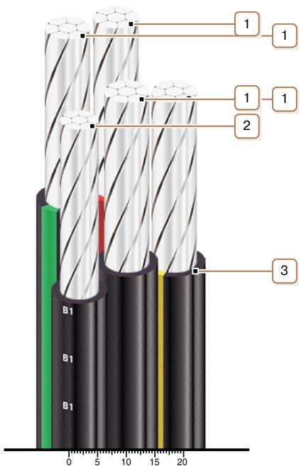
1. Aluminium multiwire compacted conductor
