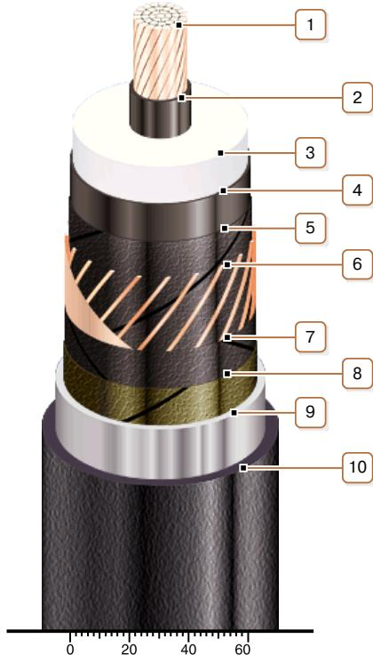
**1. Copper multiwire compact conductor**
