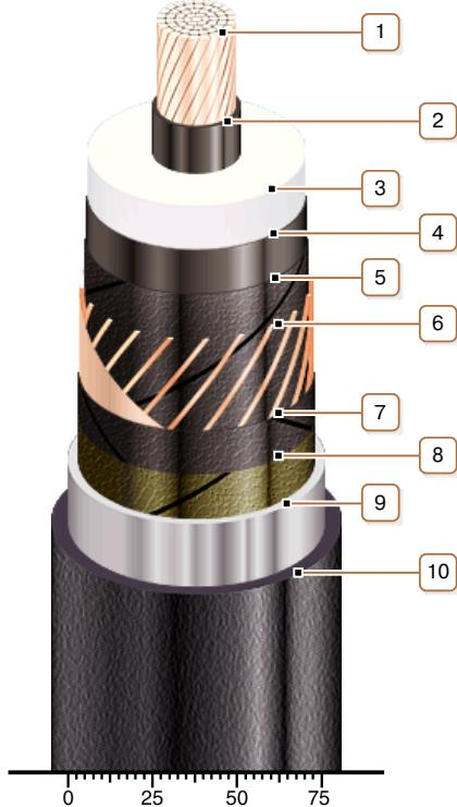
**1. Copper multiwire compact conductor**
