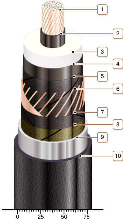
**1. Copper multiwire compact conductor**
