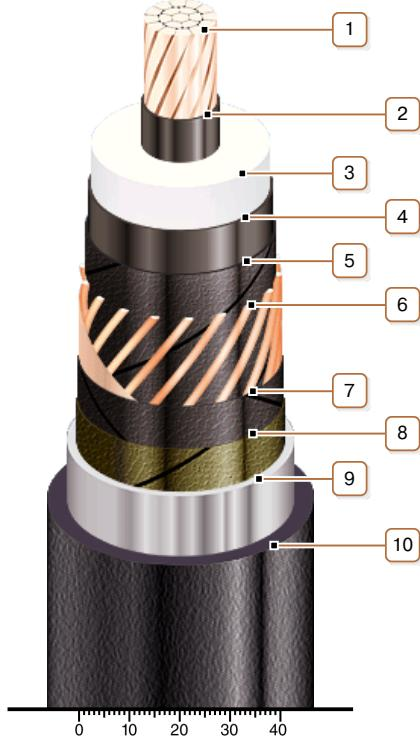
**1. Copper multiwire compact conductor**
