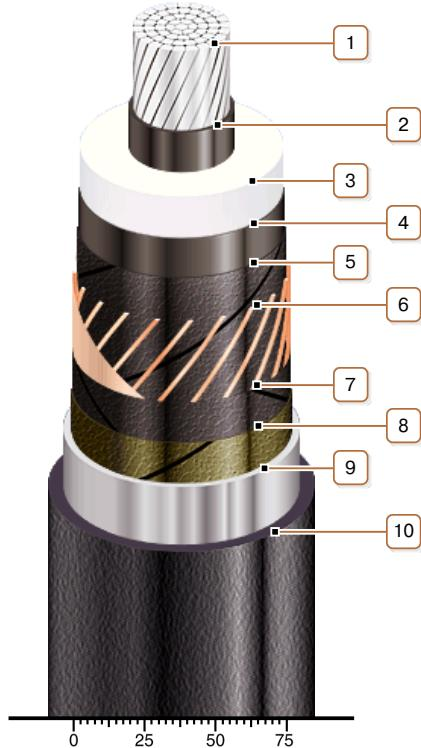
**1. Aluminium multiwire compacted conductor**
