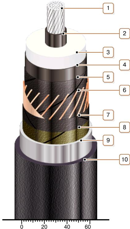
**1. Aluminium multiwire compacted conductor**
