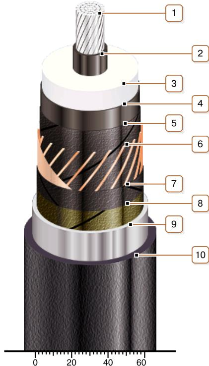
**1. Aluminium multiwire compacted conductor**
