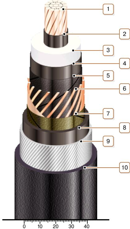
**1. Copper multiwire compact conductor**
