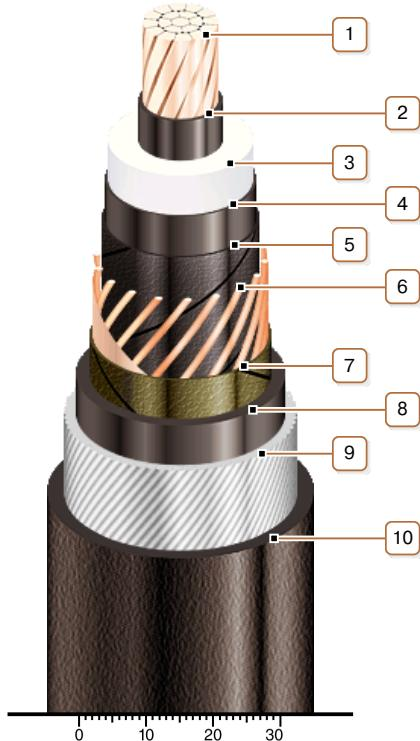
1. Copper multiwire compact conductor
