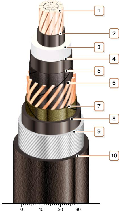
1. Copper multiwire compact conductor
