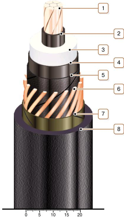
**1. Copper multiwire compact conductor**
