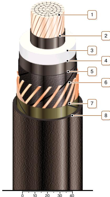
**CONSTRUCTION****1. Copper multiwire compact conductor**
