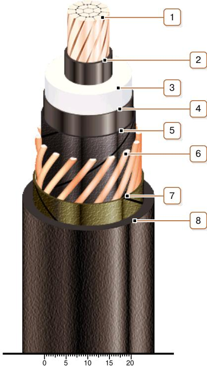
**1. Copper multiwire compact conductor***Note: It is possible to manufacture cable with sealed conductor.***2. Inner extruded semiconducting layer****3. XLPE insulation****4. Outer extruded semiconducting layer****5. Lapping layer of semiconductive swellable tape****6. Copper screen****7. Lapping layer of nonwoven cloth tape****8. PVC compound outer sheath**
