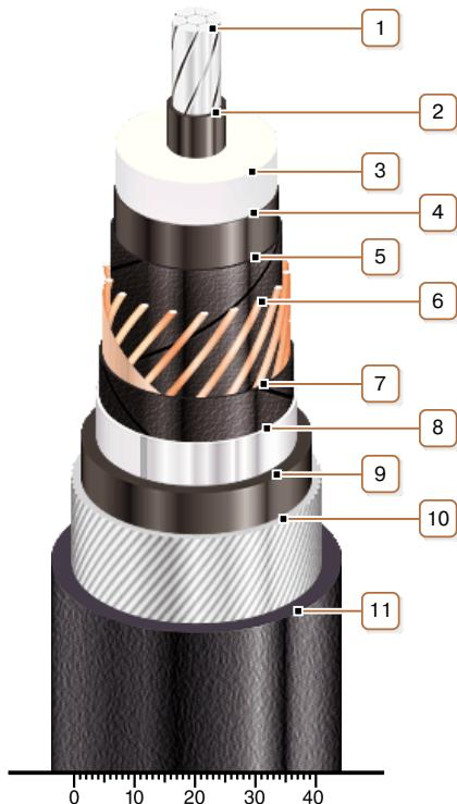
**1. Aluminium multiwire compacted conductor**
