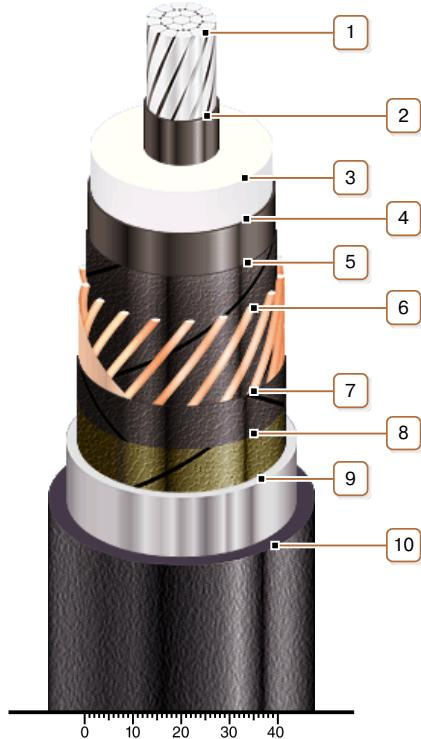
**1. Aluminium multiwire compacted conductor**
