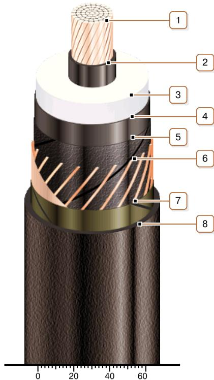
**1. Copper multiwire compact conductor**
